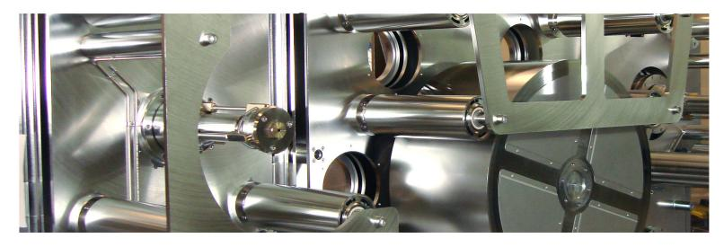
Mustang's revolutionary roll-to-roll vacuum deposition systems deposit uniform thin-film coatings onto a rolling substrate as it passes through the vacuum chamber. The thin films and other coatings (Front Contact-TCO e.g. ZnO, Window Layer - CdS, Absorber - CIGS, Back Contact - Molybdenum) are deposited by sputtering (physical vapor deposition - PVD), evaporation or chemical vapor deposition (CVD) or plasma enhanced chemical vapor deposition (PECVD).
